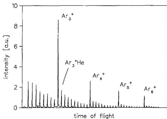
Fig. 1. Mass spectrum obtained by electron impact ionization of large helium clusters ( $\langle N \rangle \approx 7000$ ) doped with argon atoms. The photofragmentation experiment was performed on the indicated species  $Ar_3^+$  and  $Ar_3^+He$
