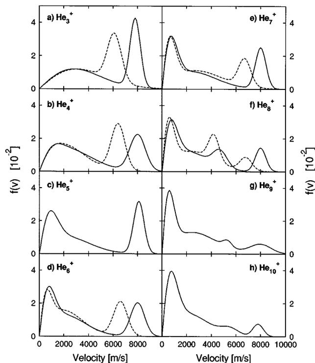
FIG. 5. Deconvoluted center-of-mass velocity distributions of the neutral fragments,  $f(v)$ , obtained from the experimental data in Fig. 4. The solid line refers to an excitation wavelength of 225 nm (5.5 eV); the dashed line to 270 nm (4.6 eV).
