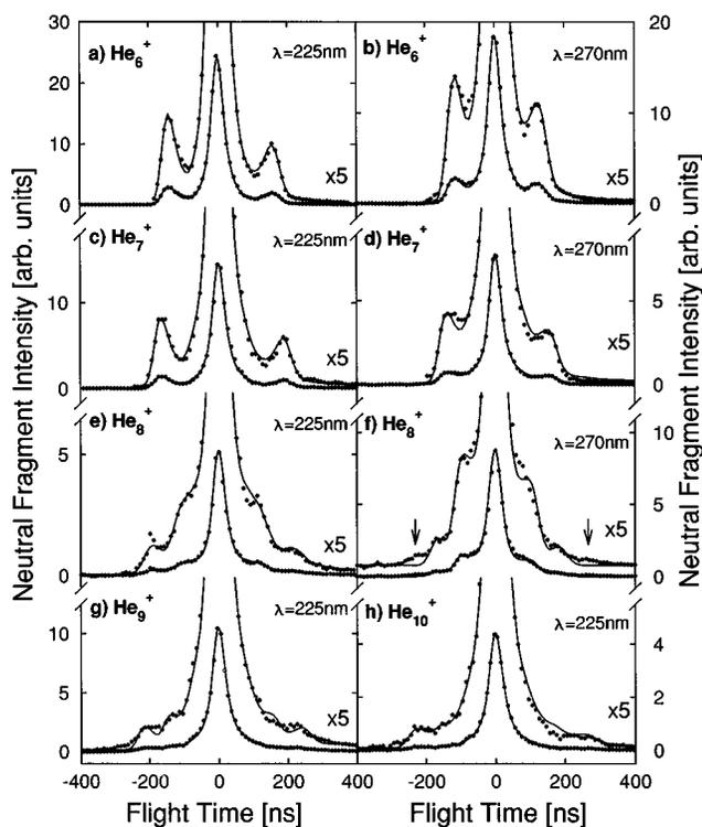
FIG. 4. Time-of-flight spectra of the neutral fragments after photodissociation of  $\text{He}_n^+$  ( $n=6-10$ ) at 225 and 270 nm with the laser light polarized parallel to the beam axis. The solid line represents the result of a fit with model functions. The small outermost pair of wings appearing at 270 nm has not been fitted here for better visibility.
