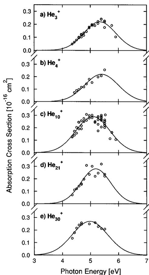
FIG. 2. Measured photoabsorption cross sections ( $\circ$ ) as a function of the laser excitation energy for (a)  $\text{He}_3^+$ , (b)  $\text{He}_4^+$ , (c)  $\text{He}_{10}^+$ , (d)  $\text{He}_{21}^+$ , and (e)  $\text{He}_{30}^+$  together with a Gaussian fit ( $\text{—}$ ) to the data. The resulting fit parameters are summarized in Table I.
