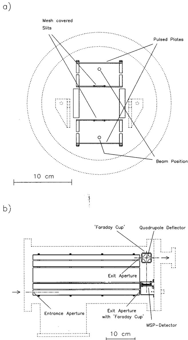
FIG. 3. Setup of the mass selector. (a) Front view; (b) side view.
