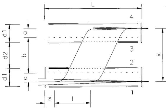
FIG. 1. Schematic of the mass selector. Short high voltage pulses applied to plates 1 and 4 are used to displace a preaccelerated convergent ion beam laterally.  $l$ : length of the ion beam package displacement,  $x$ : total displacement,  $a$ : beam offset traversed during the high voltage pulse,  $b$ : length of the field free region,  $d1/d2$ : plate separations,  $s$ : length of the portion of the ion beam which cannot be used due to field distortion,  $L$ : total length.
