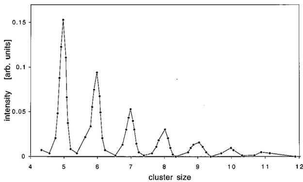
FIG. 5. Mass spectrum of ionized copper clusters  $\text{Cu}_n^+$ ,  $n=5-12$ . The spectrum was obtained by measuring the transmitted ion current for different repetition frequencies of the high voltage pulses.
