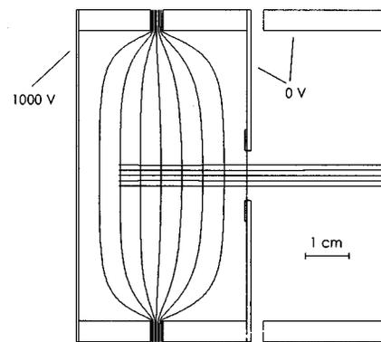
FIG. 4. Simulation (Ref. 1) of the field distribution in the acceleration region and the consequent ion trajectories. In the simulation, the field is switched off when the ions have on average gained 500 eV. The resulting trajectories deviate from perfectly horizontal trajectories by less than  $0.11^\circ$ .
