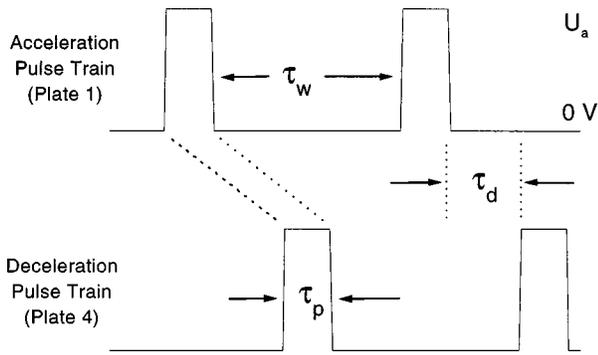
FIG. 2. Schematic of the timing of the high voltage pulses. Trains of identical pulses, displaced in time, are applied to plates 1 and 4 (see Fig. 1).  $\tau_p$ : pulse length,  $\tau_d$ : drift time between acceleration and deceleration pulse,  $\tau_w$ : time between consecutive acceleration pulses.
