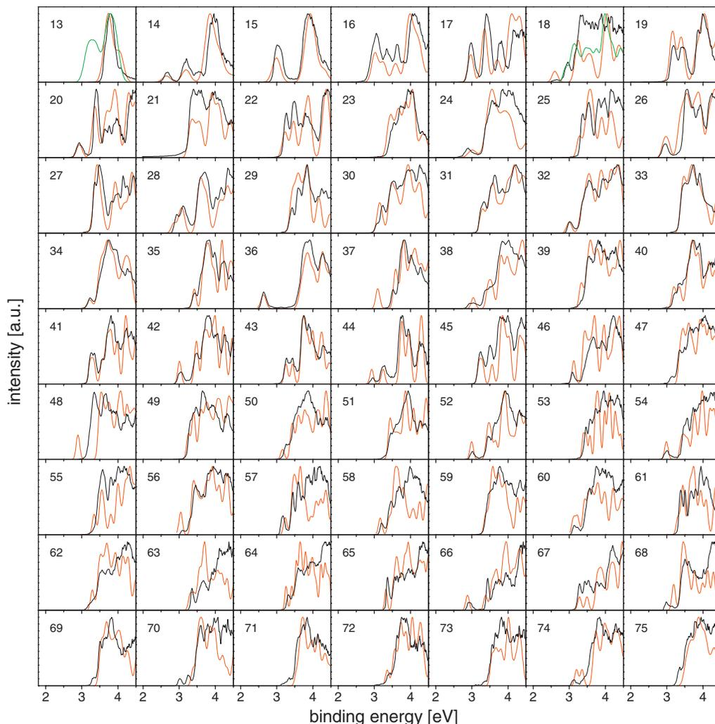
FIG. 1. Photoelectron spectra of cold ( $T=80$  K) aluminum cluster anions, measured at a photon energy of 4.99 eV (thick dark lines), in comparison with the electron DOS as calculated for the lowest energy structure found (thin red/light lines). For size  $n=13$ , the thin green (light) curve shows the DOS obtained from a decahedral isomer. For  $n=18$ , we show the DOS curves for two nearly degenerate isomers.
