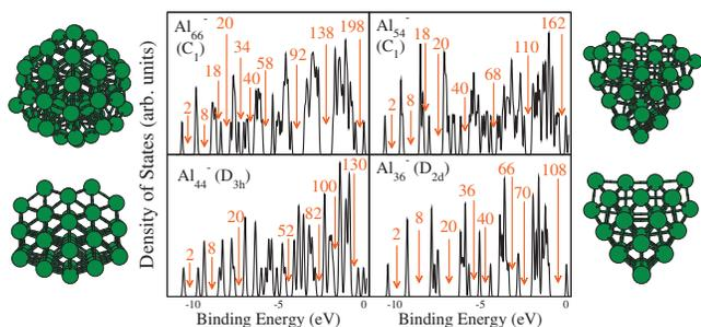
FIG. 4. Total DOS of four cluster sizes ( $\text{Al}_{66}^-$ ,  $\text{Al}_{44}^-$ ,  $\text{Al}_{54}^-$ , and  $\text{Al}_{36}^-$ ), which exhibit a large bandgap in the photoelectron spectra. The geometrical structure of the clusters is indicated.
