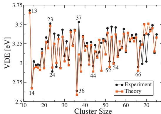
FIG. 2. The VDE of  $\text{Al}_n^-$  cluster anions is shown as a function of cluster size. The filled black points are the experimental results, and the filled red (light) squares the theoretical results. The DFT results have been globally shifted by 0.1 eV (the systematic error) in order to help the comparison.
