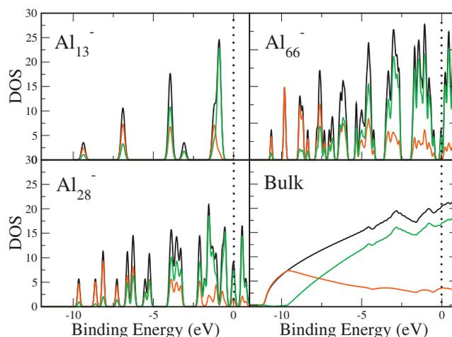
FIG. 3. The calculated total electron DOS of  $\text{Al}_n^-$  clusters and the bulk are shown by the black lines. The red and green lines indicate the partial contributions from atomic s- and p- states. The Fermi energy, shown by the dotted vertical lines, is taken as the energy reference.
