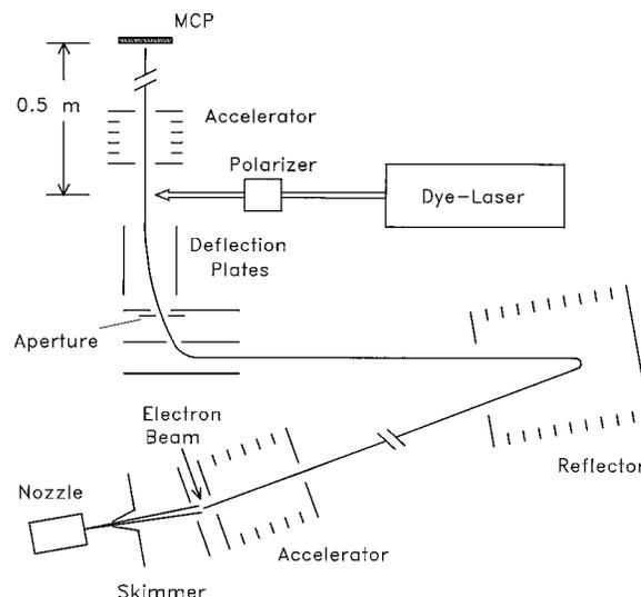
FIG. 1. Schematic diagram of the apparatus. The reflector angle of  $2^\circ$  is highly exaggerated.
