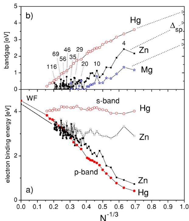
FIG. 2. (a) Energy positions of the two uppermost states visible in the photoelectron spectra of  $Hg_n^-$  and  $Zn_n^-$  clusters as a function of size. (b) Band gaps as derived from graph (a). For comparison the data for  $Mg_n^-$  (Ref. 7) is shown as well. Additionally the lowest excitation energies ( $^1S_0 \rightarrow ^3P_0$ ) of the respective atoms have been inserted; the lines serve to guide the eye.
