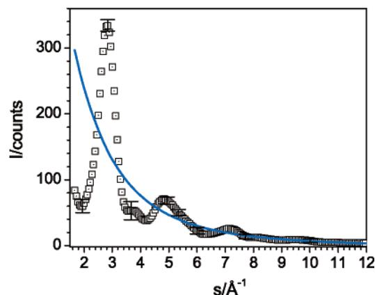
**Figure 3.** Total experimental scattering intensity,  $I_{\text{tot}}^{\text{exp}}$  (open squares), and the product of atomic and background scattering,  $I_{\text{at}}I_{\text{back}}$  (line), as a function of the momentum transfer  $s$  for  $\text{Ag}_{55}^+$ . The error bars show the standard deviation ( $\pm\sigma$ ).
