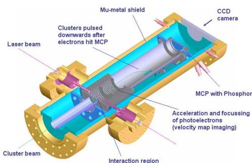
**Figure 2.** Imaging photoelectron spectrometer. The laser detached electrons are accelerated onto a multichannel plate and produce a spot pattern on its phosphor anode, which is recorded by a CCD camera. The inhomogeneous acceleration field follows the principle of velocity map imaging[8], which strongly reduces the influence of the finite ion-laser interaction volume onto the resolution of the spectrometer.
