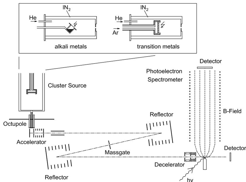
**Figure 1.** Schematic of the experimental setup. It consists of a cluster source, a thermalization radio frequency multipole ion trap, a high resolution tandem reflectron time-of-flight mass spectrometer, and a magnetic bottle type time-of-flight photoelectron spectrometer. Depending on the cluster materials in the cluster source either thermal evaporation or magnetron sputtering is applied to bring the material into the gas phase. See text for details.
