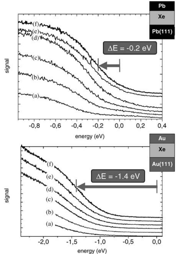
**FIGURE 9** (top) Fermi edges for different amounts of lead on 60 ML xenon/Pb(111). The small shift can be explained due to the cluster charging energy  $E_C$  because of  $\Delta\Phi \approx 0$ . (bottom) Fermi edges for different amounts of gold on 60 ML xenon/Au(111): (a) 0.7 ML, (b) 1.0 ML, (c) 1.4 ML, (d) 1.7 ML (e) 2.1 ML and (f) 2.4 ML. The large shift is at least partly explained due to static charging (for details see text)
