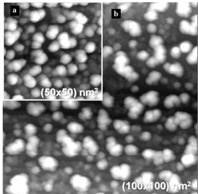
**FIGURE 2** STM images ( $T = 5$  K) for 3.6 ML Au on 10 ML Xe/Pb(111) (a) STM image before Xe desorption,  $\approx 206$  clusters per  $10^4 \text{ nm}^2$  ( $U_T = 1.3$  V,  $I_T = 10$  pA) (b) STM image after Xe desorption,  $\approx 204$  clusters per  $10^4 \text{ nm}^2$  ( $U_T = 1.5$  V,  $I_T = 20$  pA)
