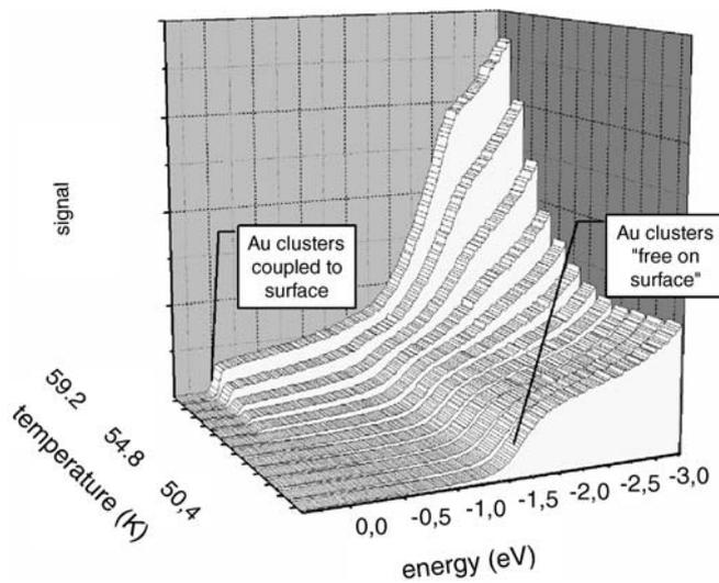
**FIGURE 5** Change of the UPS spectra for Au Clusters on 60 ML Xe/Pb(111) during controlled heating of the sample from 50 K to 60 K with a rate of 0.2 K/min. One observes a constant decrease of the shifted Fermi edge of Au clusters on xenon until it vanishes completely, while the Fermi edge of the Pb substrate and of the clusters coupled to the substrate arise at the reference Fermi energy of 0 eV
