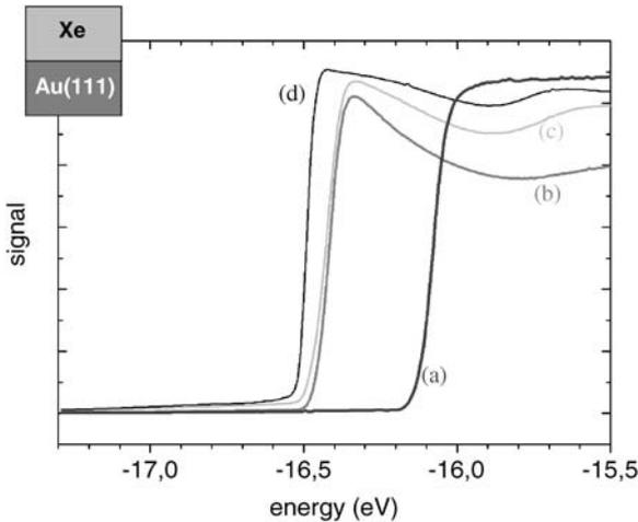
**FIGURE 8** Lower cut-off energy of the UPS spectra: (a) pristine Au(111) substrate, (b) 10 ML Xe/Au(111), (c) 30 ML Xe/Au(111) and (d) 160 ML Xe/Au(111). The spectra are scaled to similar maximum signal for better visualization. A bias voltage of  $-5$  eV was applied to the sample. The energy scale is given by the Fermi energy  $E_F = 0$  eV
